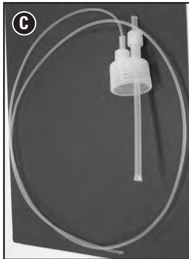
Figure 1. Methyl mercury distillation system: (A) entire system, (B) distillation, (C) distillation vessel cap, and (D) receiving vessel cap.
